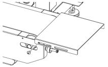
**3** Fix the table with the two screws out of three screws removed at the procedure 1. Please refer to the illustration on the right for the detail.
