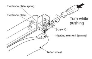
How to replace fusing type heating element (For Fi, FiK-600 fusing types)
