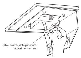
The pressure adjusting spring is installed inside the screw.
