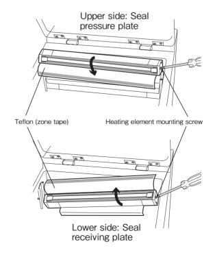
When inserting the heating element, insert each terminal between electrode plate and electrode plate spring.
