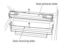
When the seal receiving plate is removed, you will see the tube below it. As in the illustration on the right (1), lift up the pin holding the tube with hands to your side (2). Slide off the tube base toward you (3) and remove the tube.
