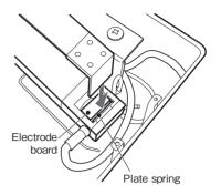
Make sure that the heating element stays in place with the electrode as you securely tighten the screw to keep the heating element in place.
